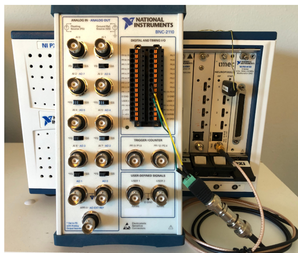
Figure 5 – (A) Example JSON file describing the wiring of the BNC breakout box. In this example the 1s square wave pulse from the PXI chassis is relayed to the first digital channel (P0.0). The next two digital channels are used to record timestamps of licks and camera frames. The first analog channel is used to record a continuous signal from a breathing sensor. (B) A picture of the BNC breakout box (BNC-2110, National Instruments) which receives the synchronization pulse from the PXI chassis as an input in the first digital channel (P0.0). Picture credits Open Ephys .
