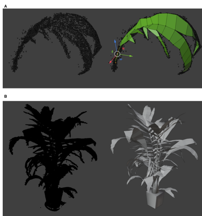
Figure 5 - 3D reconstruction from LiDAR point clouds. A) Building plane meshes on point cloud with the poly build tool of Blender. B) Full reconstruction of the 3D mock-up from points cloud.
